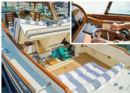
The center cockpit seats electrically lift to reveal a large storage area as well as easy access to mechanical systems. Inset: The uncluttered helm has all the controls within reach.
